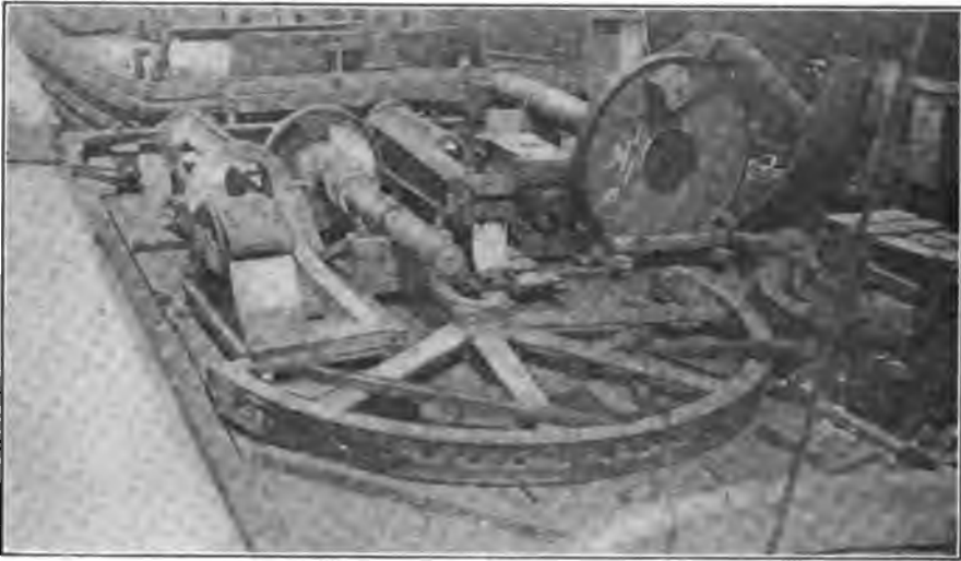
FIG. 148.—Parts of 18-in. \times 42-in., 22-in. \times 36-in. and 30-in. \times 60-in. Corliss engines for shipment to the Philippine Islands. Note skidding and cradles for crank-shafts; boxing around crank-pin; protection at ends of pillow-blocks; and skidding and crating of cylinder.
